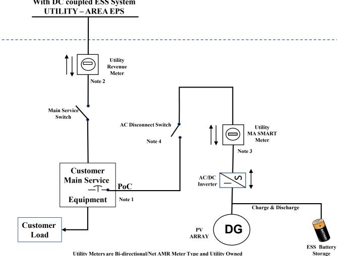
Meter Locations determined by Utility for Service Access Requirements
